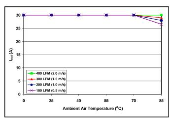
Figure 9: Maximum output power derating curves vs. ambient air temperature for airflow rates of 100 LFM through 400 LFM with air flowing across the converter from input to output (24V input).
