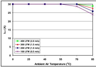
Figure 7: Maximum output power derating curves vs. ambient air temperature for airflow rates of 100 LFM through 400 LFM with air flowing across the converter from pin 3 to pin 1 (48V input).
