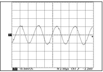
Figure 19: Input reflected ripple current,  $i_{s}$ , through a 10  $\mu H$  source inductor at nominal input voltage and rated load current (10 mA/div). See Figure 17.
