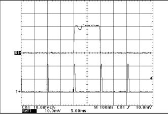
Figure 22: Load current (20A/div) as a function of time when the converter attempts to turn on into a 10 m $\Omega$ short circuit. Top trace (5ms/div) is an expansion of the on-time portion of the bottom trace.
