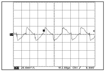
Figure 20: Output voltage ripple at nominal input voltage and rated load current (20 mV/div). Load capacitance: 1µF ceramic capacitor and  $10\mu F$  tantalum capacitor. Bandwidth: 20 MHz. See Figure 17.
