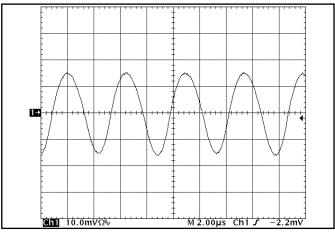
Figure 18: Input Terminal Ripple Current, ic, at full rated output current and nominal input voltage with  $10\mu H$  source impedance and  $47\underline{\mu}F$ electrolytic capacitor (500 mA/div). See Figure 17.
