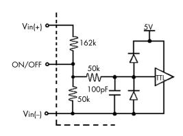
Figure B: Internal ON/OFF pin circuitry
