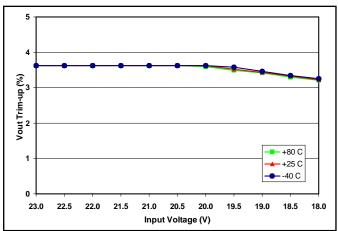
Figure 27: Achieveable trim-up percentage vs. input voltage at +85°C, +25°C and -40°C (all at full load). Full trim-up percentage is achieved at loads of 50% or less across full temperature and input voltage range.
