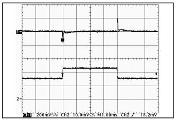
Figure 15: Output voltage response to step-change in load current (50%-75%-50% of Iout(max);  $dI/dt = 0.1A/\mu s$ ). Load cap:  $10\mu F$ ,  $100\ m\Omega$  ESR tantalum cap and 1µF ceramic cap. Ch 1: Vout (200mV/div), Ch 2: Iout (10A/div).
