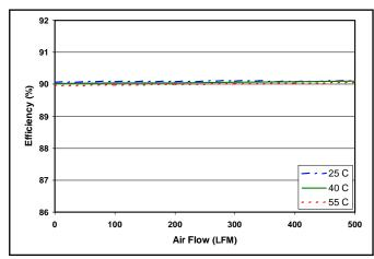
Figure 2: Efficiency at nominal output voltage and 60% rated power vs. airflow rate for ambient air temperatures of 25°C, 40°C, and 55°C (48V input).
