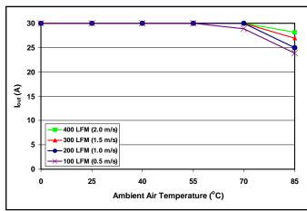
Figure 11: Maximum output power derating curves vs. ambient air temperature for airflow rates of 100 LFM through 400 LFM with air flowing across the converter from input to output (48V input).
