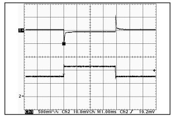
Figure 16: Output voltage response to step-change in load current (50%-75%-50% of Iout(max):  $dI/dt = 5A/\mu s$ ). Load cap: 470 $\mu F$ , 30 m $\Omega$  ESR tantalum cap and 1µF ceramic cap. Ch 1: Vout (500mV/div), Ch 2: Iout (10A/div).
